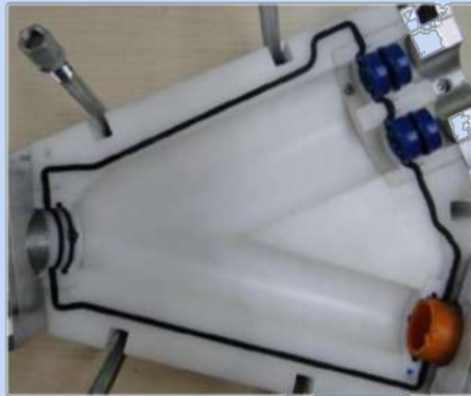
MONTAGING O-RINGS TO THE TOOL(bottom side)
