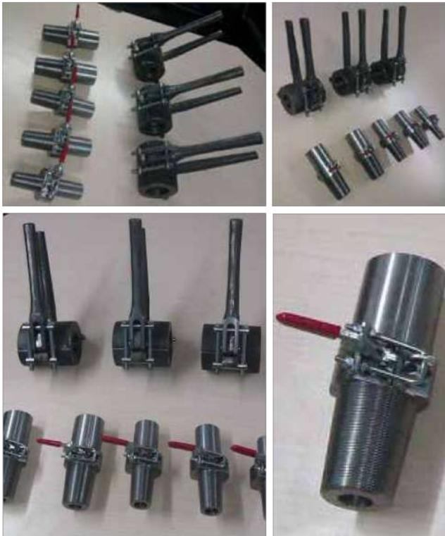
There are two disadvantages of standard plastic pipe coupling devices for people who are blowing cable. One of them is coupling two pipes together takes too much time and the other one is you cannot take out plastic pipe coupling device after cable blowing inside the coupling device. You can take it out only by cutting it, which means that you can use it only once.
