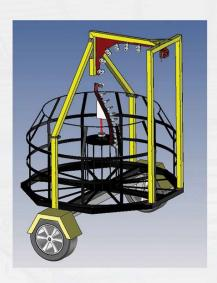
The Trailer Mounted Cable Fleeter replaces the manual handling for "figure eighting" cable and gives extra protection and security to the cable. Following deployment of the cable in the first leg of duct route the balance of the cable is taken out from the drum and took care of into the Fleeter, thereby delivering the cable end ready for blowing into the second leg.
